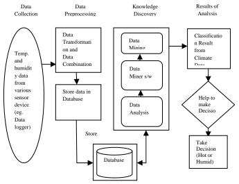
Fig. 3 Design of Temperature and Humidity Data Analysis System
